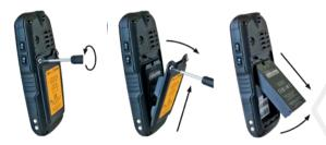
» Loosen the screws on the battery compartment using the Screwdriver provided.
